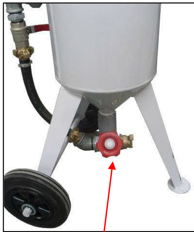
Media flow control valve
